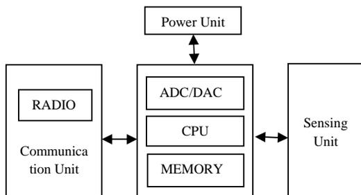
Fig 1: Wireless Sensor Network Architecture
