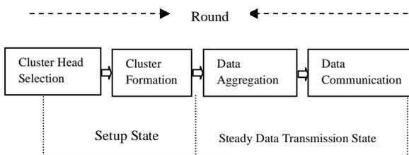
Fig 2: The composition of one round of the clustering process.
